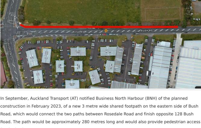
construction in February 2023, of a new 3 metre wide shared footpath on the eastern side of Bush Road, which would connect the two paths between Rosedale Road and finish opposite 128 Bush for the hockey centre patrons. Initially there were plans to also add yellow lines along the corresponding 280 metres of Bush Road,
